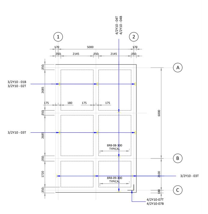
Raft Foundation Reinforcement Scale 1:75
