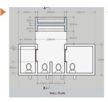
An offset lined pit means that the toilet seat is not directly above the leach pit (marked by X in the picture) – therefore the child cannot fall in. The offset pit can be shallower and can be emptied with a shovel, no expensive pump out required. Because the pit is offset, nappies cannot be thrown in easily which stops it from filling up too quickly. The pour flush design allows staff to flush with grey water, which is a sustainable and sanitary solution for drought stricken areas.
